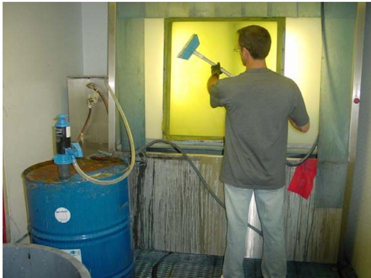
“A sealed, contained system is ideal when dealing with a toxic, flammable, or corrosive liquid,” says Grubbe. “With sealed devices, like GoatThroat pumps, you can maintain a controlled containment from one vessel to another.”
